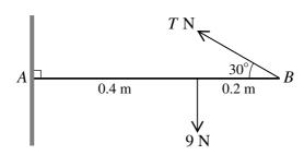
A non-uniform rod AB, of length 0.6 m and weight 9 N, has its centre of mass 0.4 m from A. The end A of the rod is in contact with a rough vertical wall. The rod is held in equilibrium, perpendicular to the wall, by means of a light string attached to B. The string is inclined at  $30^{\circ}$  to the horizontal. The tension in the string is T N (see diagram).
